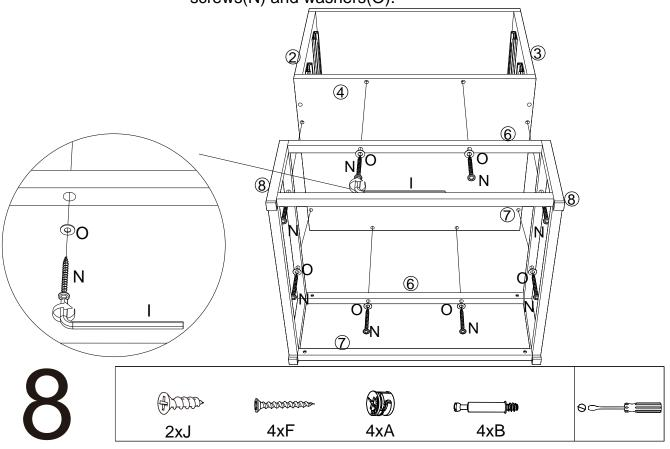
STEP 8: Assemble the top drawer as shown in below diagram using screws(J), screws(F),cam locks(A) and cam bolts(B).
